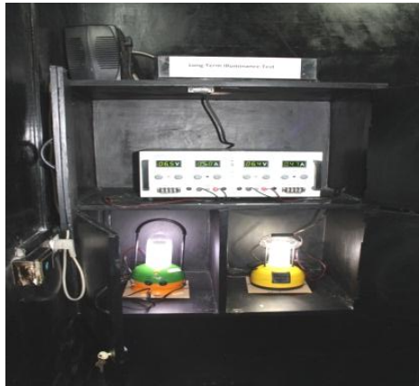
Fig. 2 Photographs of test setup used in long term illuminance test
