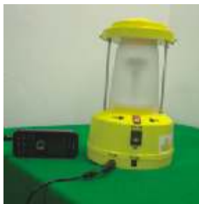
Figure 11 Inserting the mobile charging cord in the mobile the 'mobile phone charging socket'.
