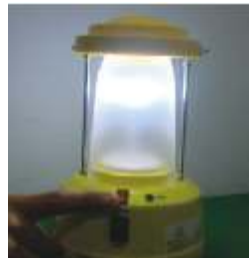
Figure 8 Controlling the brightness/dimming of the lantern
