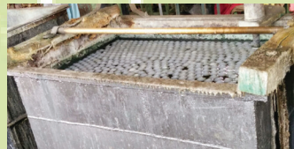
PP balls on hot process tank solution
