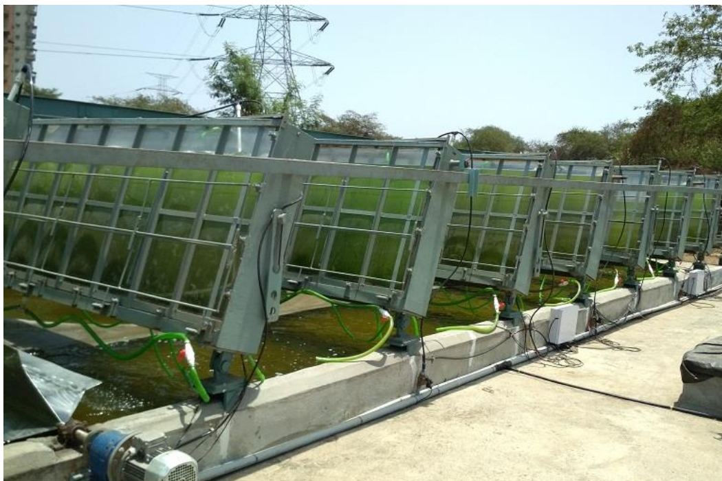
Marine algal production system in Mumbai (220 sq. meter/100,000 L)
