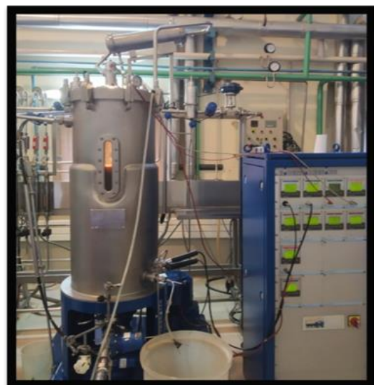
Scale up of biohydrogen production from acid pretreated water hyacinth hydrolysate in 150 liter bioreactor
