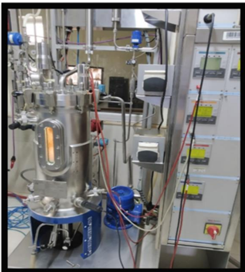
Scale up of biohydrogen production from acid pretreated water hyacinth hydrolysate in 30 liter bioreactor
