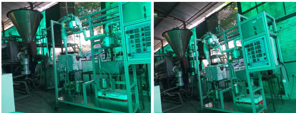
Fig. 2: TERI's 2-Stage Catalytic Cracking and Pyrolysis Vapor Upgrading Unit
