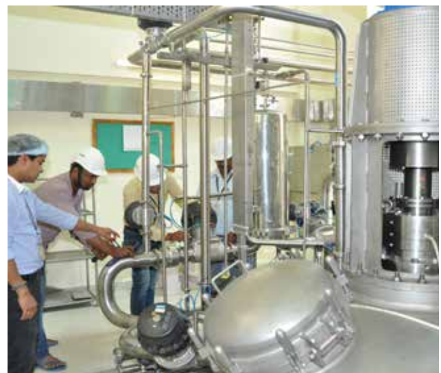
► Fermenter (15,000 litre capacity) at FTRC, TERI Gram
