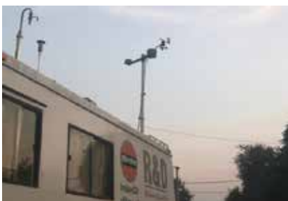
» Air quality monitoring at a roadside using Indian Oil Corporation's air quality monitoring mobile van for TAQIITA project
