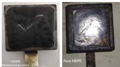
» Char formation of neat HDPE and nanocomposites
