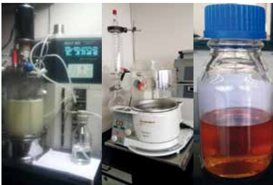
A process for microbial production and downstream purification of 2,3 butane diol from the fermentation broth (fermented by Enterobacter cloacae ) was developed by TERI.
