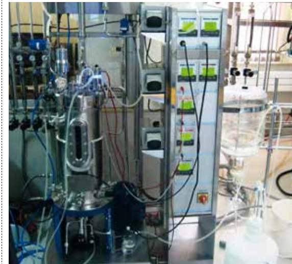
Fermentative biohydrogen production by C5 sugar utilizing Enterobacter cloacae DT-1 strain (isolated by TERI) from lignocellulosic biomass sugar (second generation feedstock) in 30 litre pilot scale bioreactor (20 litre working volume), through dark fermentation route.
