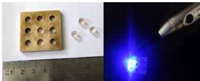
Light-cured sample along with brass mould used to prepare the sample and LED curing light to carry out the photo polymerization
