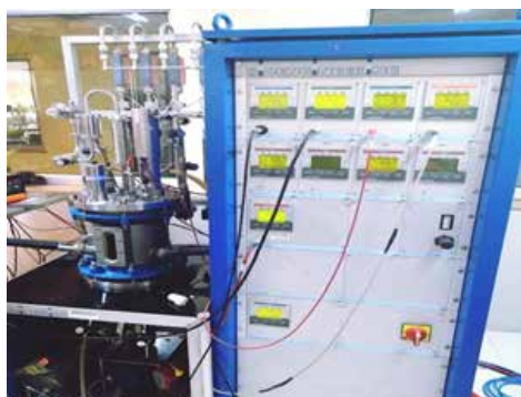
Scale up of bioethanol production process 13.5 L bioreactor
