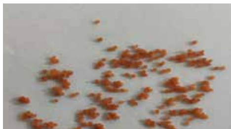
Sericin grafted encapsulated NPK fertilizer beads for controlled and sustained release of NPK fertilizer
