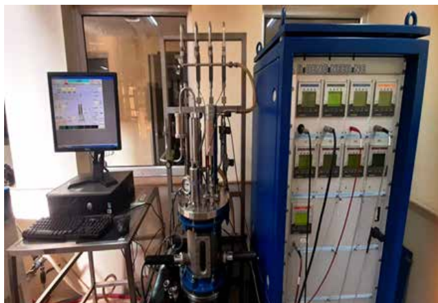
2,3 butane diol production process was up scaled in 13.5 L bioreactor
