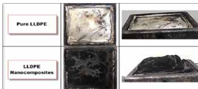
Char formation of neat LLDPE along with nanocomposites
