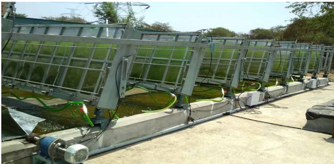
Marine algal production system in Mumbai (220 m 2 /100,000 L)
