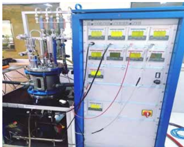
Scale up of bioethanol production by an industrial grade sugar/sugar cane black strap molasses novel yeast isolate; Candida tropicalis strain TERI DC
