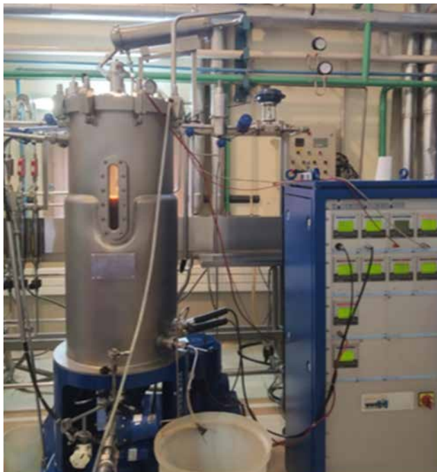
Scale up of biohydrogen production from acid pre-treated water hyacinth hydrolysate in 150 litre bioreactor
