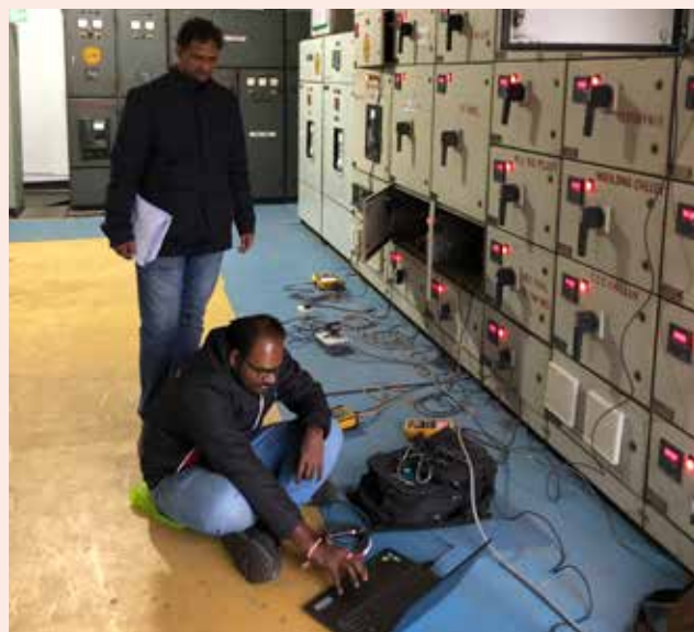
Power quality study for chilling plant with ALM 32 instrument at Dabur Nepal Private Limited
