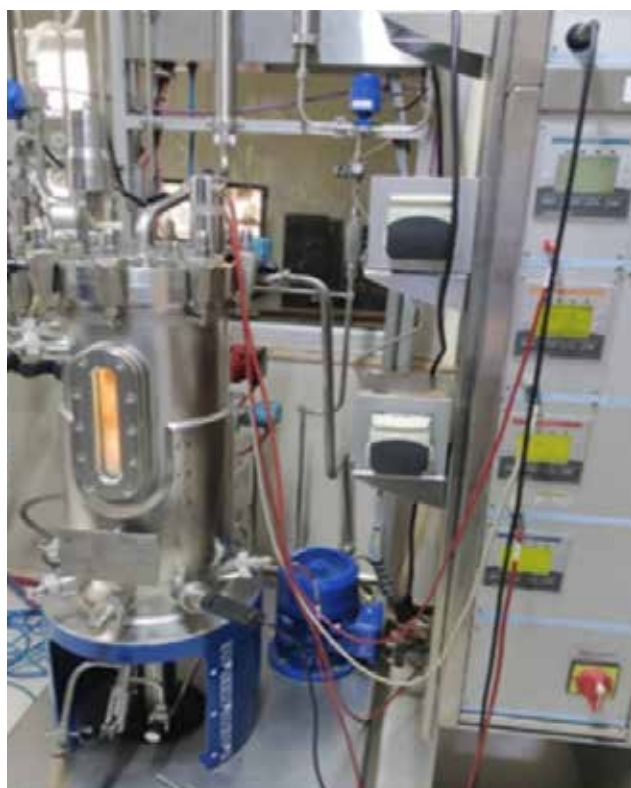
Scale up of biohydrogen production from acid pre-treated water hyacinth hydrolysate in 30 litre bioreactor
