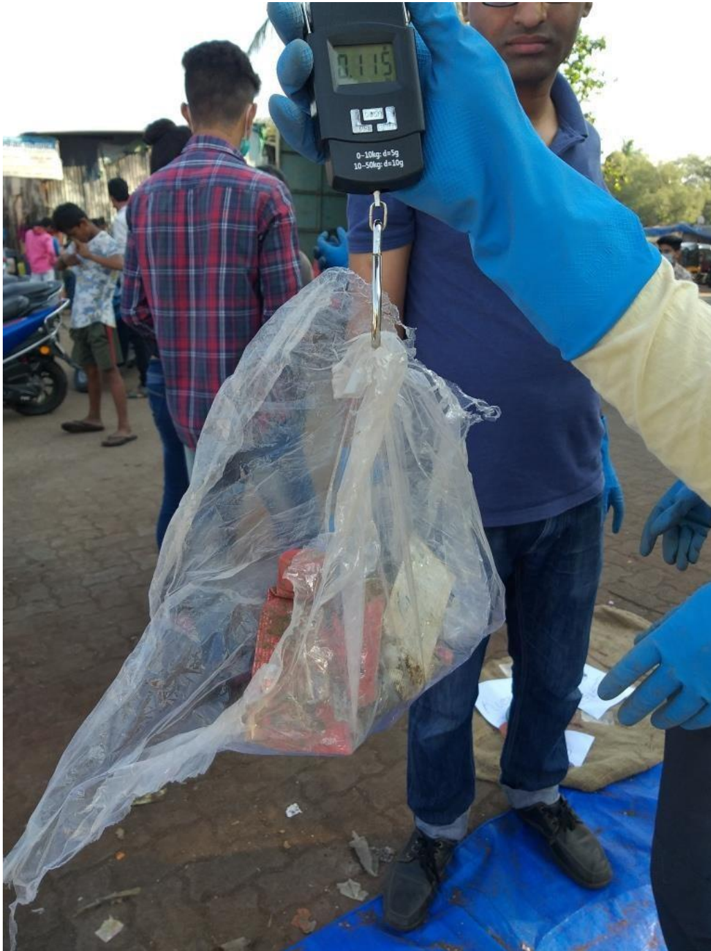
Picture No. 14: The segregated waste in different categories was weighed on the digital scale for the study.
