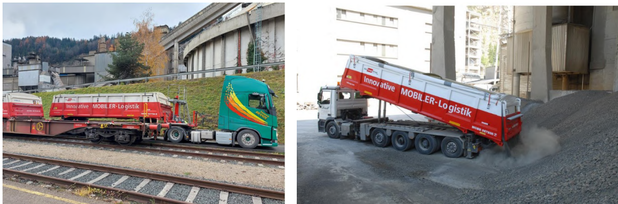
Figure 63: Swap body wagons for loose commodities
