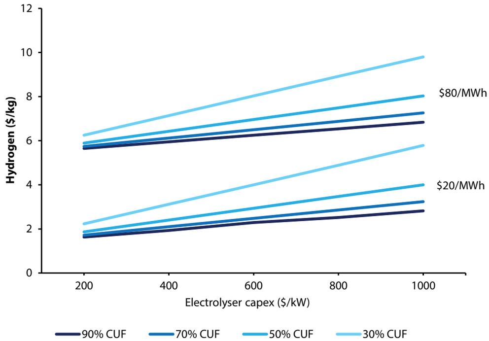
**Figure 52:** Impact of varying capacity utilization factors on cost of hydrogen
