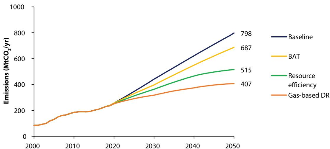
Figure 45: Emissions impact of coal to gas switch in DR facilities, 2000–50
