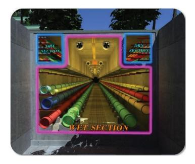
FIGURE 20 Utility tunnel, showing wet and dry sections<sup>9</sup>
