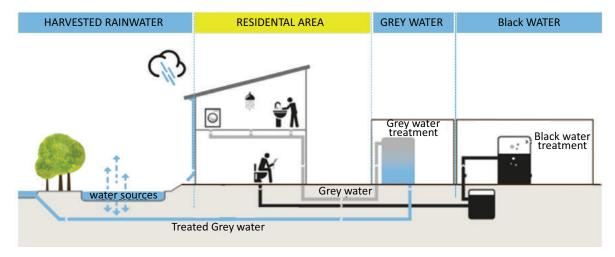
FIGURE 38 Separate waste treatment plants installed at the facility to treat grey and black water separately
