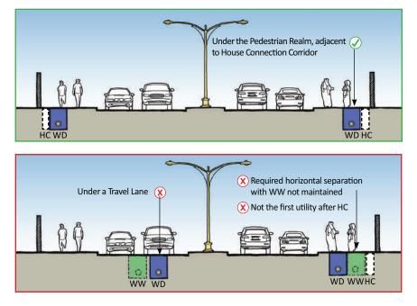
FIGURE 15 Typical potable water corridors' locations
