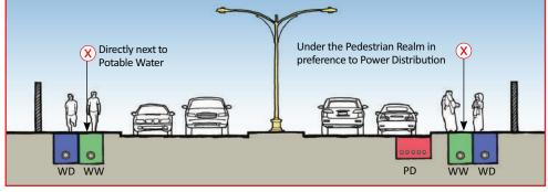
FIGURE 16 Typical wastewater collection corridors' location
