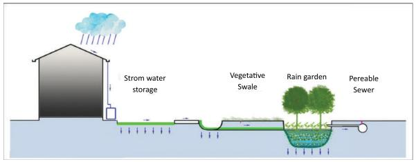
FIGURE 49 Various methods for channelizing storm water on site
