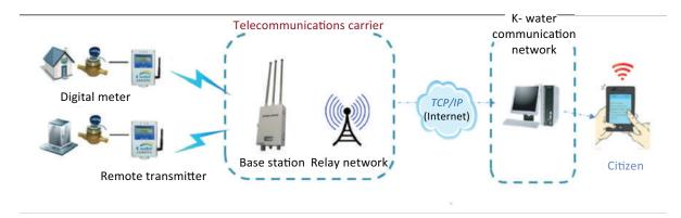
FIGURE 12 Outline of smart metering system in Seosan city<sup>2</sup>
