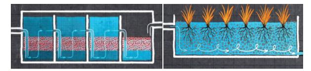
FIGURE 41 A typical gravity-fed ECO STP design, developed by Mr Tharun Kumar, Founder, ECOSTP Technologies Private Limited<sup>®</sup>
