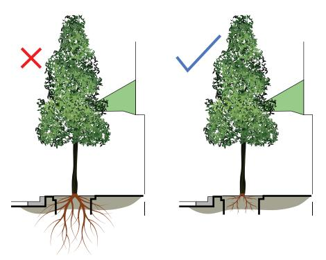
FIGURE 29 Trees with shallow root system should be planted on the podium
