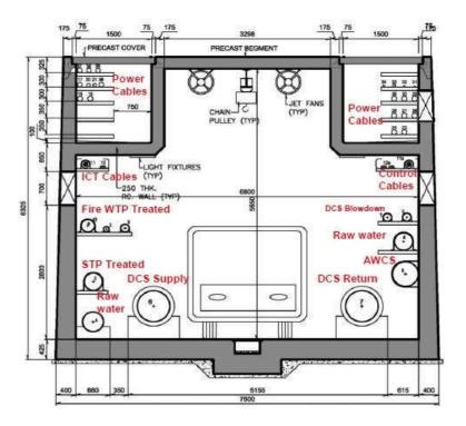
FIGURE 21 Utility tunnel, showing dimensions
