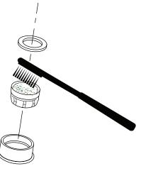
FIGURE 24 Cleaning of a water faucet aerator using a brush
