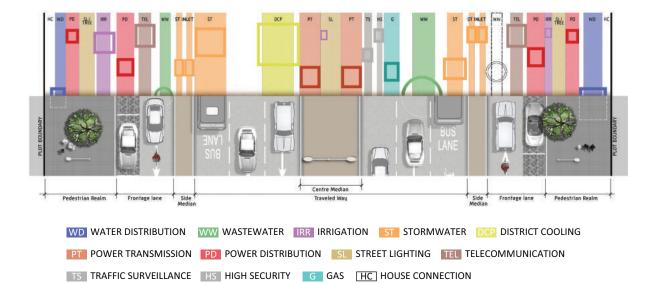
FIGURE 14 Typical utility corridor layout according to Utility Corridors Design Manual (UCDM)<sup>5</sup>
