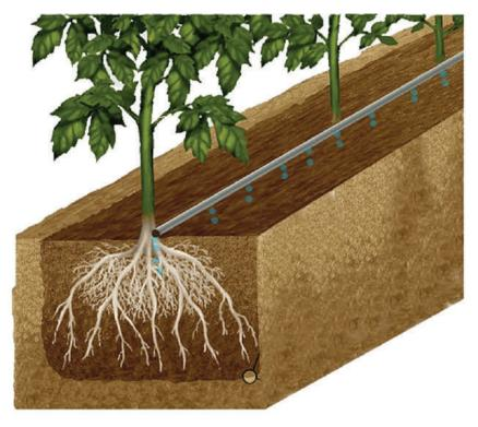
FIGURE 31 A typical drip irrigation system being used for watering the plants
