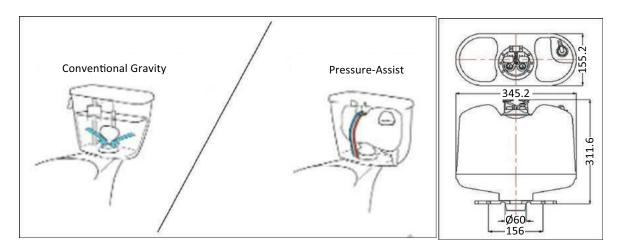
FIGURE 8 Pressure-assisted versus conventional gravity-fed flushing system with plan details of pressureassist tank
