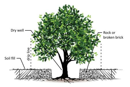
FIGURE 25 Section of a dry well constructed to protect existing tree on site
