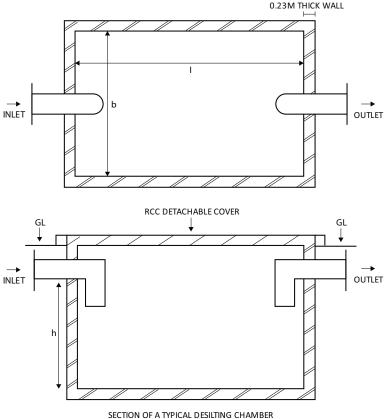
FIGURE 48 Plan and section of a typical desilting chamber
