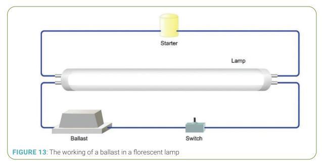
characteristics must precisely match the electrical requirements of the lamps it operates.
