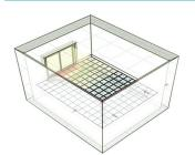
In-office buildings windows of height, 1.2 m or more in the centre of a bay with sill level at 1.0 to 1.2 m above the floor and in residential buildings windows of height 1.0 m to 1.1 m with sill height as 0.7 m to 0.9 m above the floor are recommended for good distribution of daylight indoors. Window width can accordingly be adjusted depending upon the required fenestration percentage of the floor area.
