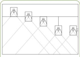
**FIGURE 16**: Mounting options for downlights: recessed, semi-recessed, surface, pendant and wall mounting
