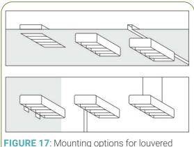
luminaires: recessed ceiling, surface, mounting on tracks, walls, floor-standing or pendant mounting
