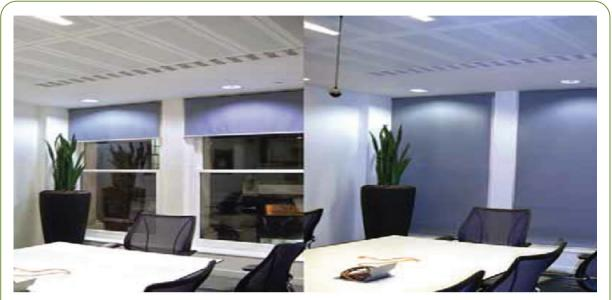
**FIGURE 6**: Comparison of the room with blinds raised and lowered showing the effect of changing the window wall reflectance
