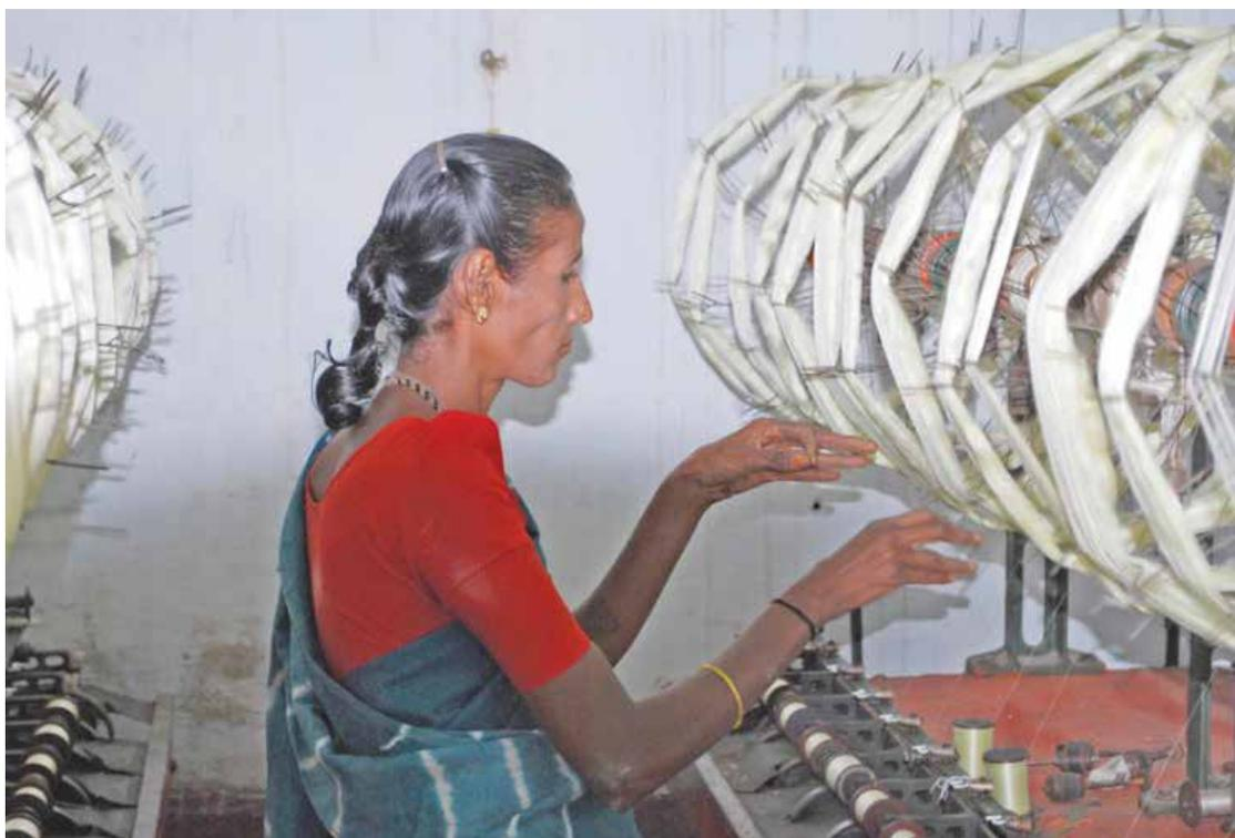
**FIGURE 4:** Silk thread twisting process
