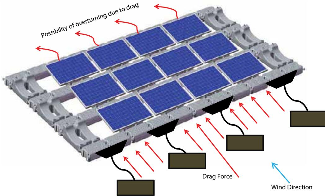
**Figure 24:** Schematic of drag forces developed in floating solar PV plant
