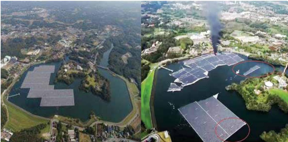
**Figure 25:** Japan's 13.7MWp floating solar PV plant before (A) and after (B). The red circle indicates that the anchoring and mooring line remained intact
