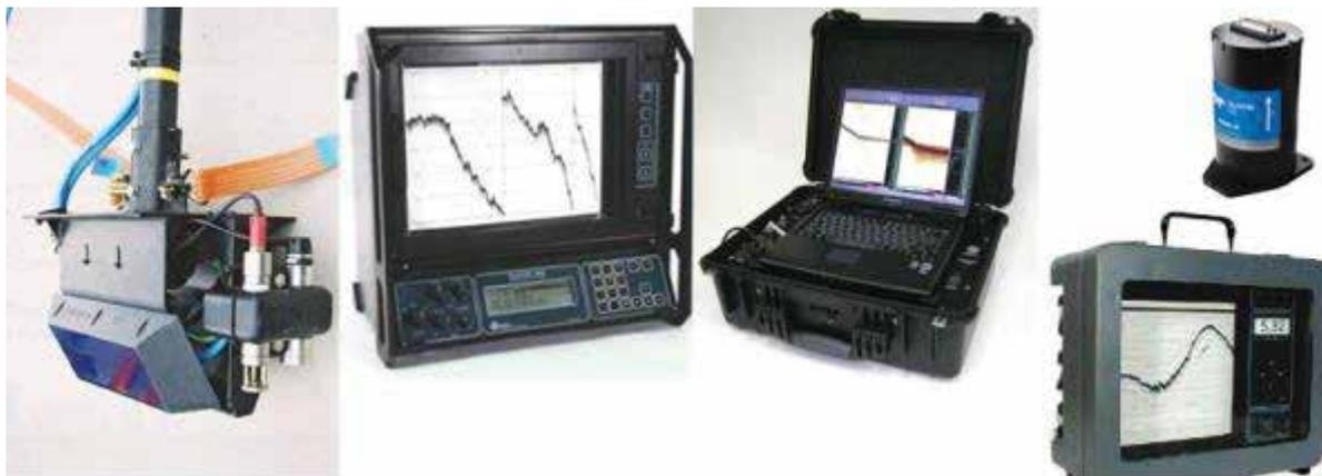
**Figure 22:** Instruments for conducting bathymetric/hydrographic surveys
