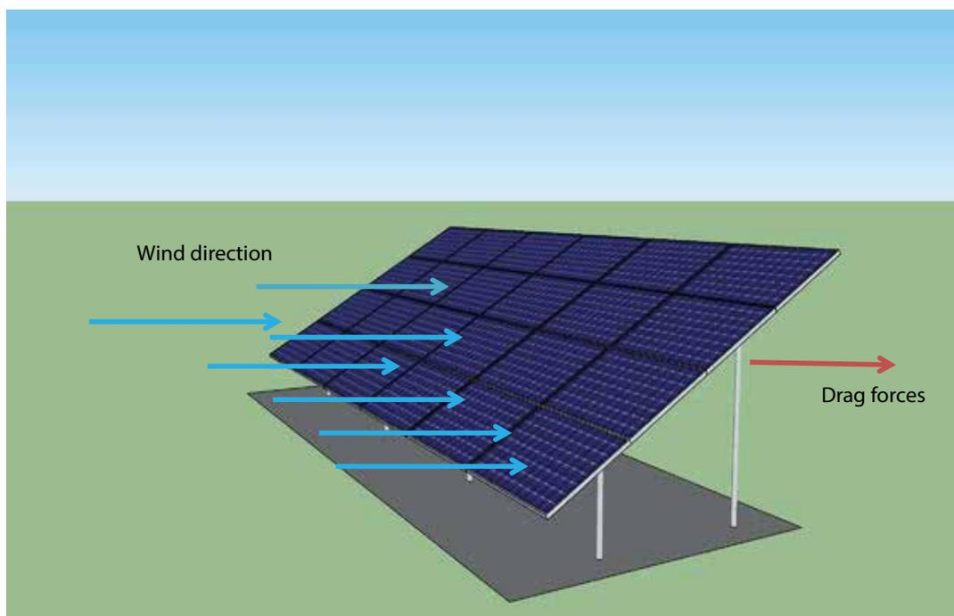
**Figure 23:** Drag forces in ground-mounted solar PV (only for representational purpose)
