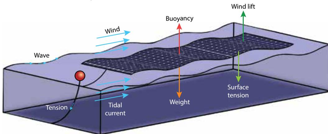
**Figure 17:** Schematic of forces on submerged FSPV plant
