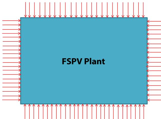
**Figure 26:** Drag forces on floating solar PV plant (a representational image)
