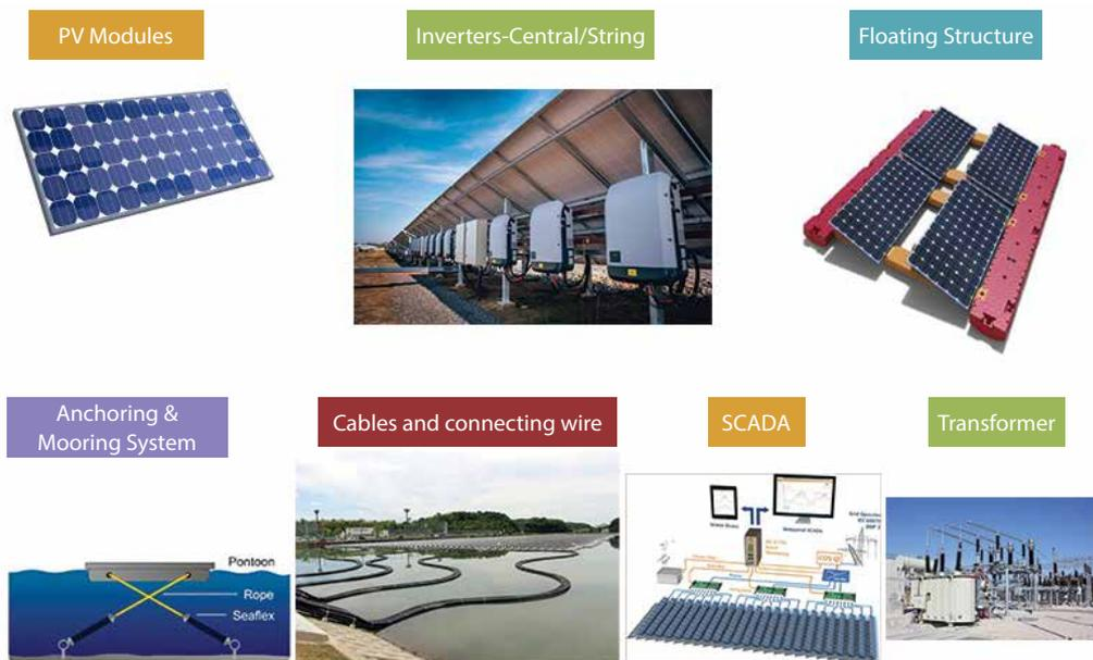
**Figure 2:** Major components of floating solar PV
