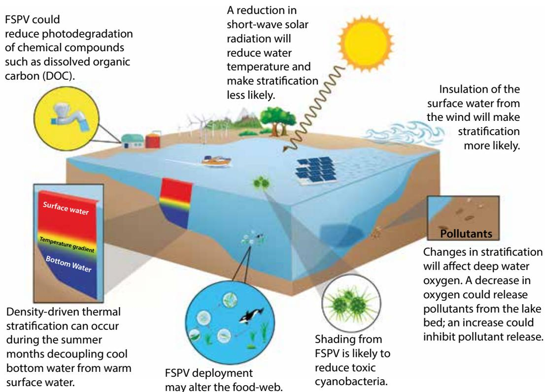
**Figure 19:** Potential impact of deploying large-scale floating solar PV
