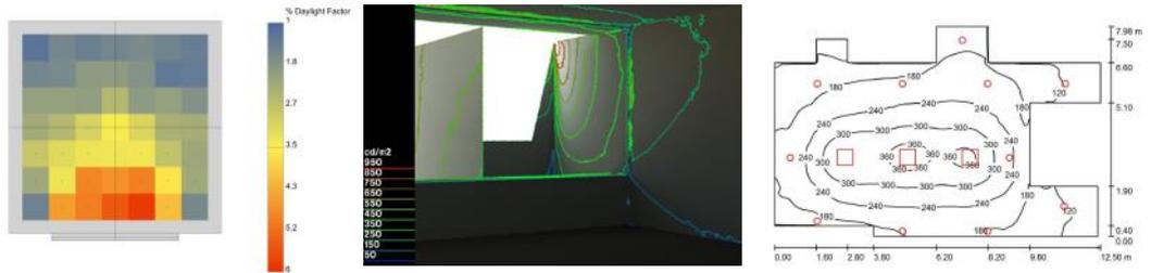
Daylight inside a building depends entirely upon the design of the building, orientation, opening design, shading, internal arrangements etc. The session will cover definitions and concepts for daylight integration, calculations for Daylight Factor (DF), useful daylight illuminance (UDI), Daylight Autonomy (DA) and hand holding exercises. Various green building certifications in India have requirement for daylight integration, these will be explained along with handholding exercises.
