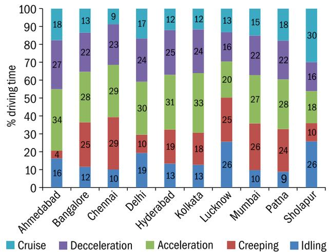
**Figure 6:** Percentage of driving time spent by cars in different driving conditions in 10 cities.
