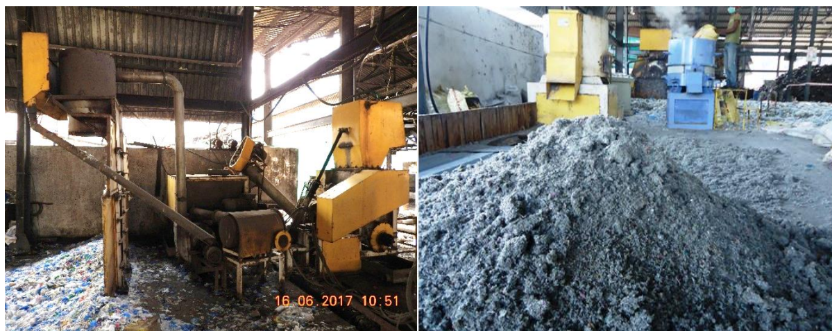
Picture No. 18: Plastic Baling machine (Left) and Plastic agglomerate (right) at Turbhe landfill site
