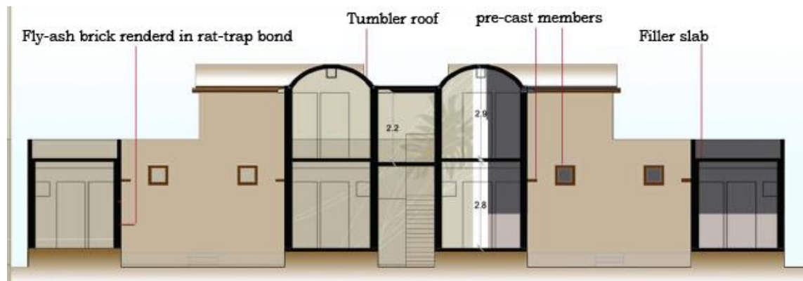
Figure7.47: Section displaying construction techniques used
