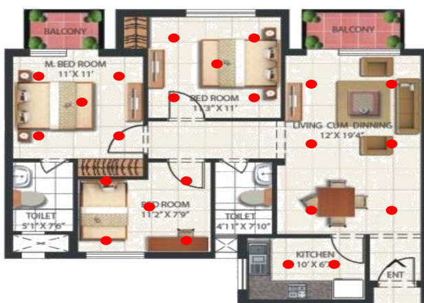
Figure8.14: Lux level measurement grid
