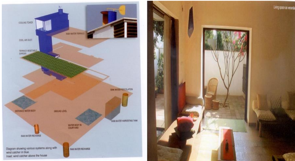
Figure 3.13: Diagram showing various systems along with wind catcher in blue
