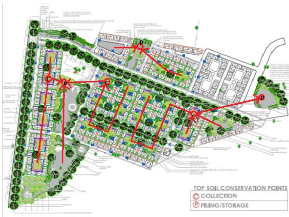
Figure7.44: AutoCAD drawing showing top soil collection and storage points
