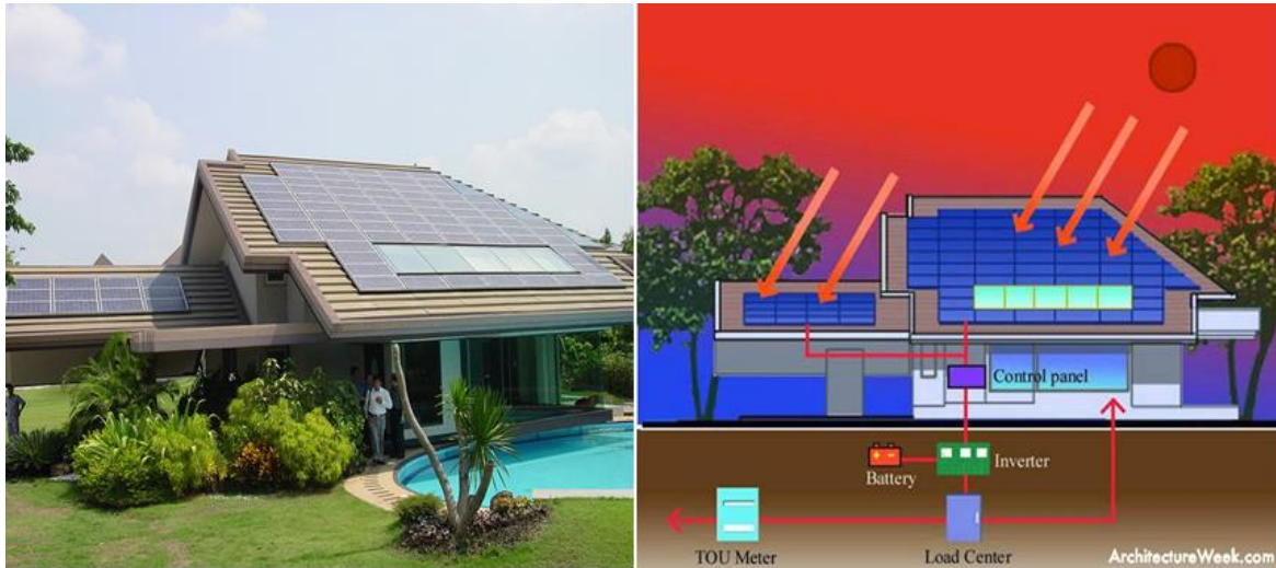
Figure 3.24: Left- Bio solar house as seen from front, Right- Detail of PV solar system installed in house.
