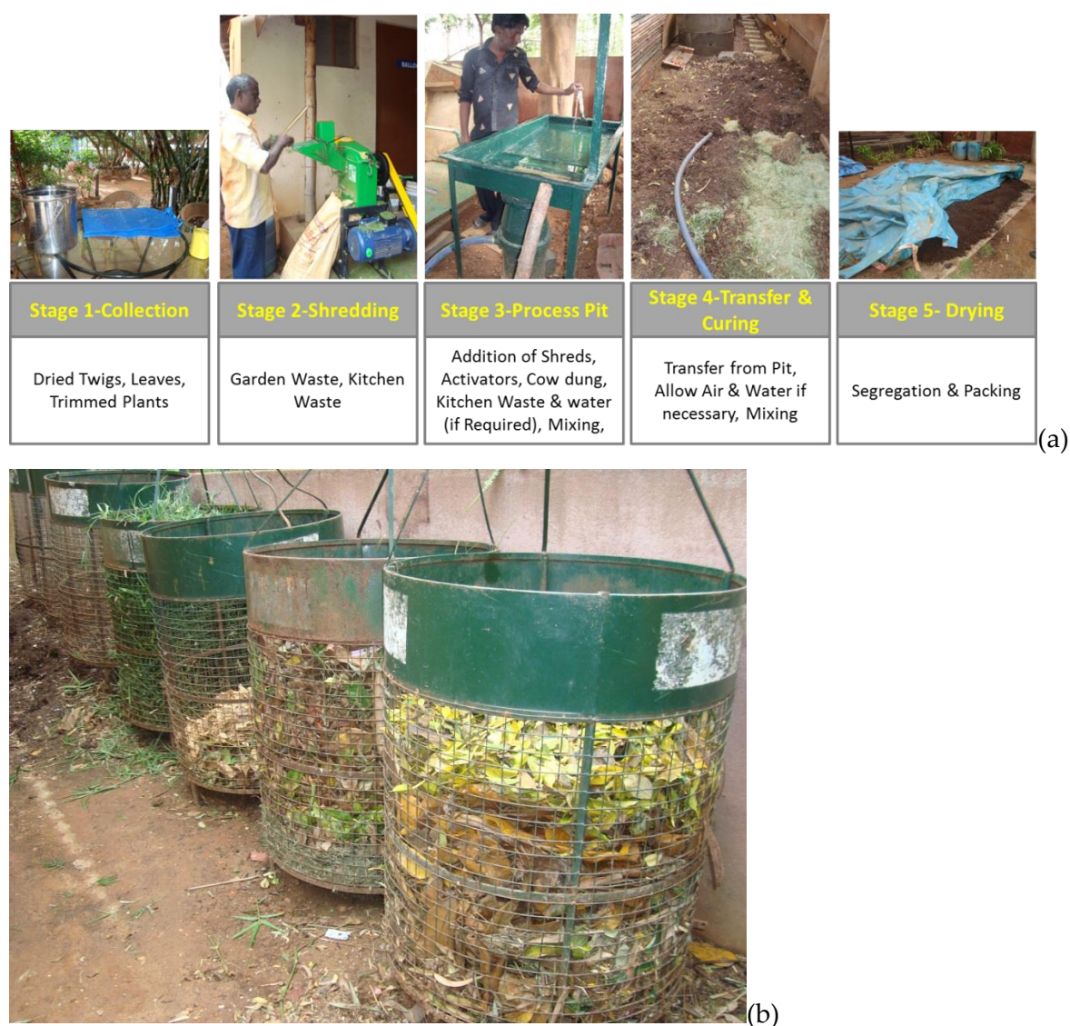
Figure 4.47: (a) Stage wise process for composting ; (b). Bins Provided for Leaf composter
