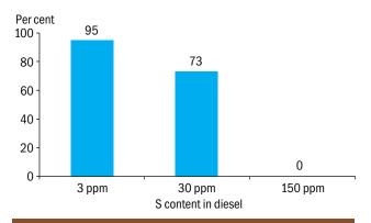
**Figure 11:** PM removal efficiency of a DPF using different quality of fuels *Source:* ICCT (2012)
