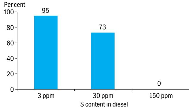
**Figure 11:** PM removal efficiency of a DPF using different quality of fuels
