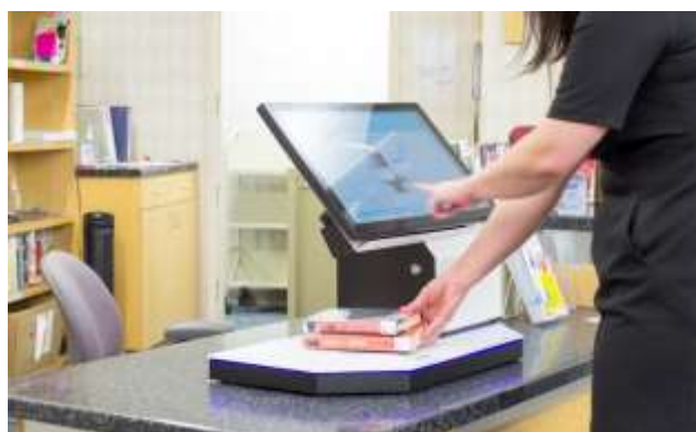
Figure 4. RFID work station by using biometric authentication
