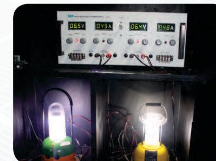
Long-term Illuminance Test Setup
