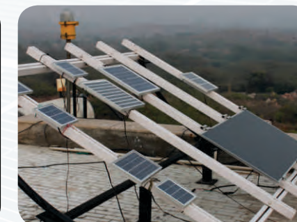
Outdoor Solar Module Test Setup
