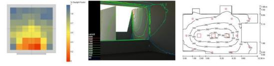
Daylight inside a building depends entirely upon the design of the building, orientation, opening design, shading, internal arrangements etc. The session will cover definitions and concepts for daylight integration, calculations for Daylight Factor (DF), useful daylight illuminance (UDI), Daylight Autonomy (DA) and hand holding exercises. Various green building certifications in India have requirement for daylight integration, these will be explained along with handholding exercises.
