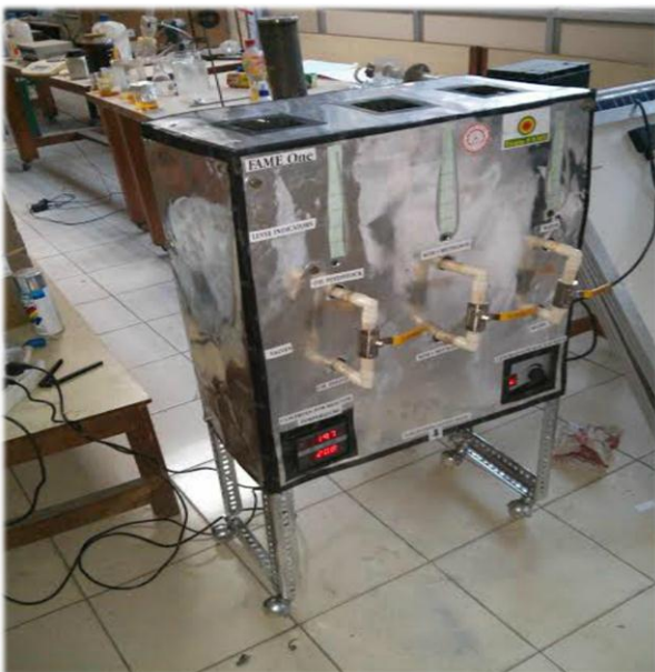
Figure 5: Machine made by IIT students that converts Waste cooking oil to Bio-fuels
