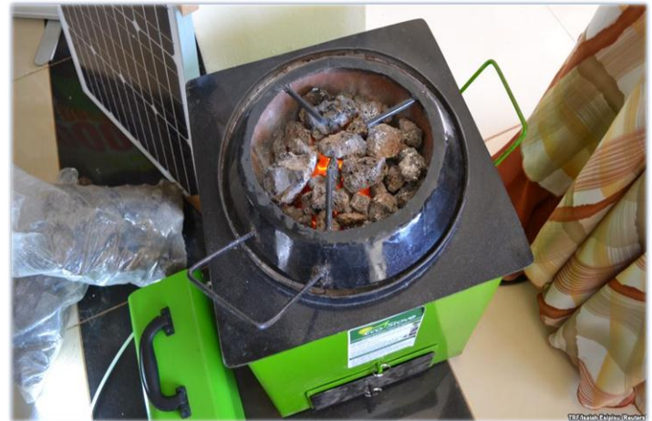
Picture 1: Volcanic rock stove built by the Eco Group Limited
